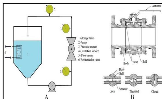
Hydrodynamic cavitation was generated using an in-house constructed unit termed the Hydrocavitator which has a feed vessel tank with maximum capacity of 25 L and operates in a re-circulation mode. Effluent from the feed tank is pumped using a triplex plunger pump (SPECK NP25) with a maximum discharge pressure of 4,500 psi and passes through an orifice unit (orifice area about  $7.0 \times 10^{-2} m^2$ ) followed by a catalyst bed and
