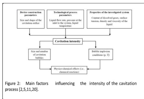
The first group consists of parameters such as the size and shape of the cavitation inducer and the flow chamber which determine the structural characteristics of the reactor
