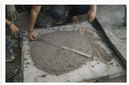
Measuring diameter of spread (mm)
